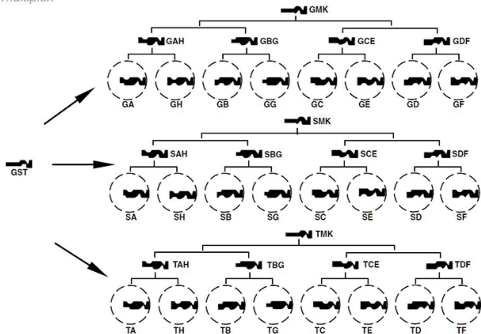
**Note:** The section of the key is determined by viewing the key from the bow towards the tip.
