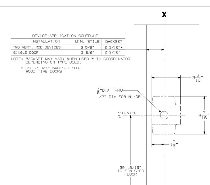
REMOVE GLASS STOP HEAD OR BEAD IN AREA OF DEVICE IF REQUIRED
