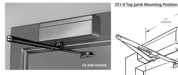
Top Jamb applications - The 351 closer is mounted on the frame face above the door. The foot is mounted on the push side of door. This application is for use on exterior doors opening out to protect the closer from the weather.
