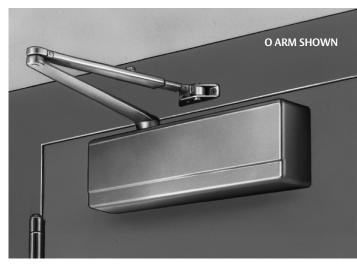
The standard application of the 351 door closer is the most common and the most desirable. The closer mounts on the hinge (pull) side of door (except when the W Corner Bracket is used). **Note:** This application is not recommended on exterior doors (the closer is not protected from weather). The cover projection normally limits the door opening to a maximum of 160°.
