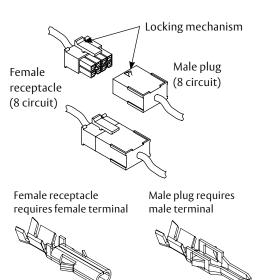
The plug and receptacle connectors are designed to mate and lock together as shown in the figure. Plug the connectors onto each other with the locking mechanism aligned as indicated.
