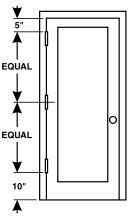
The top of the top hinge should be 5" from the jamb header.
