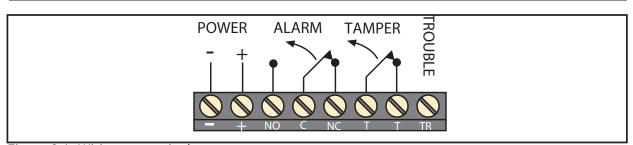
Figure 3.1: Wiring to terminals
