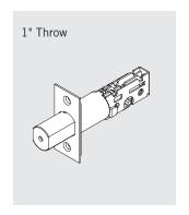
26170 — 1-1/8"  $\times$  2-1/4" front, 1" diameter, 1" throw dead bolt with 2-3/8"—2-3/4" adjustable backset. Square corner. Standard for DB600 Series. 26171 — 1-1/8"  $\times$  2-1/4" front, 1" diameter, 1" throw dead bolt with 2-3/8"—2-3/4" adjustable backset. 1/4" radiused corner. Optional for DB600 Series. 26173 — 1" diameter, 1" throw dead bolt with 2-3/8"—2-3/4" adjustable backset. Drive in. Optional for DB600 Series.
